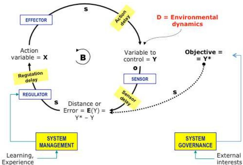
**Figure 8. Standard Model of a one-lever Control System (Mella, 2014, p.49)**
